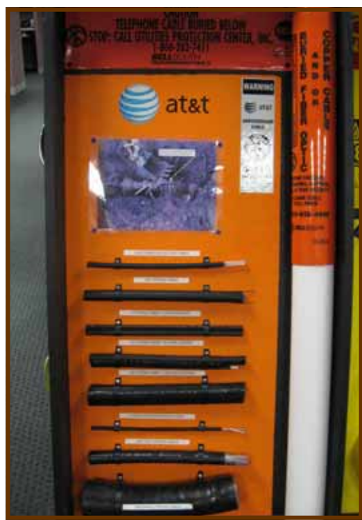
Different kinds of underground cable on display.
